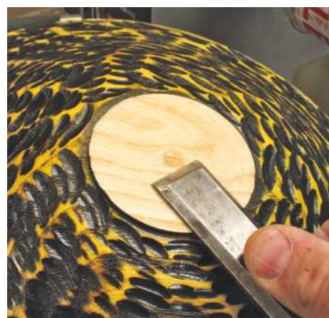
▲ Pic.33 Remove the last bit by hand with a skew chisel. Doing it slightly at an angle to the grain means that you are not digging into the surface of the base
